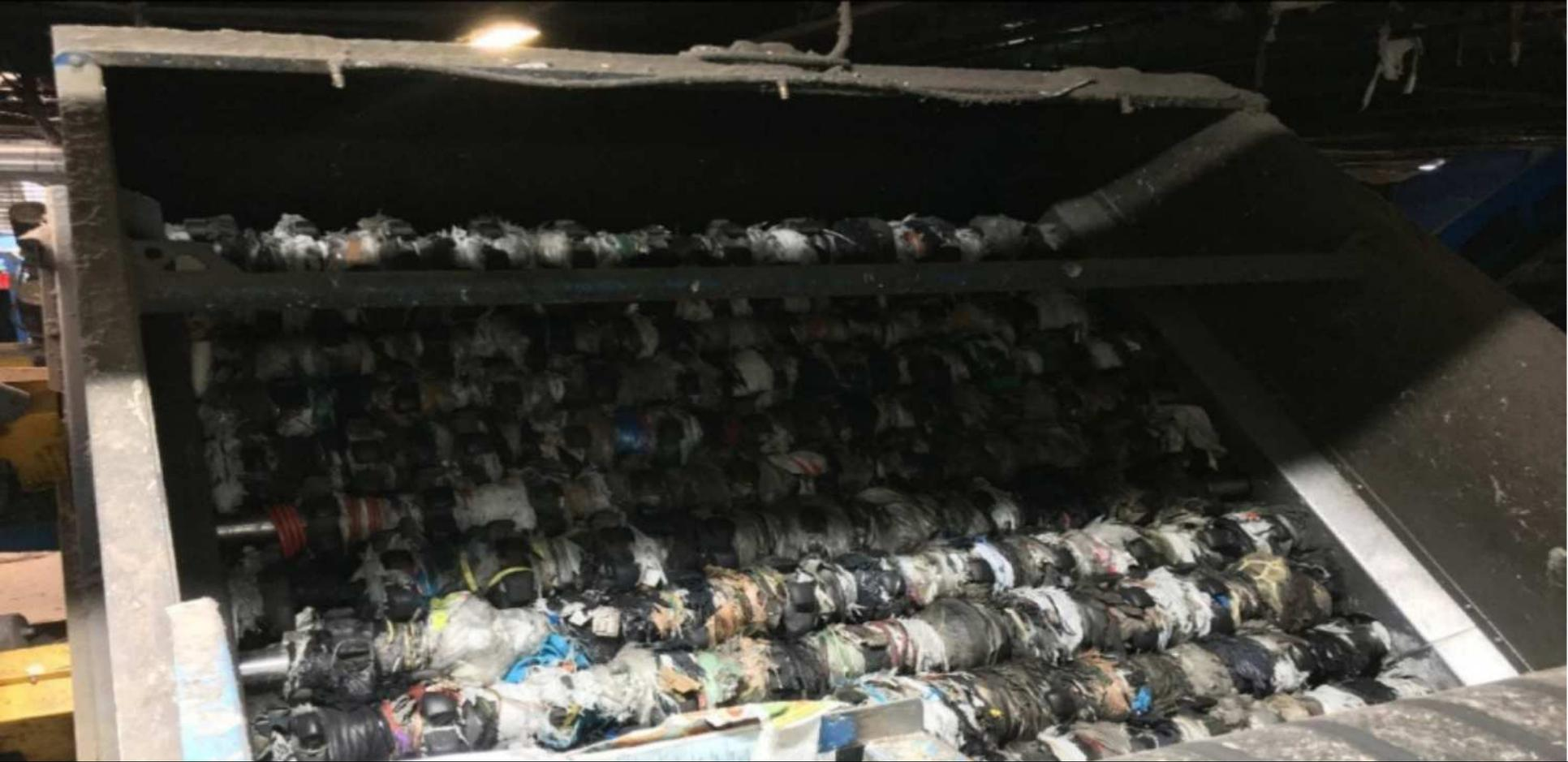
Plastic bags wrapped around equipment at the Materials Recycling Facility, causing damage to equipment and hazards for employees.
